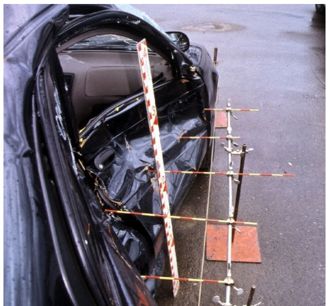
Figure C3 Side of a Post-FMVSS 214 Passenger Vehicle after Collision with a SUV (Sport Utility Vehicle)
