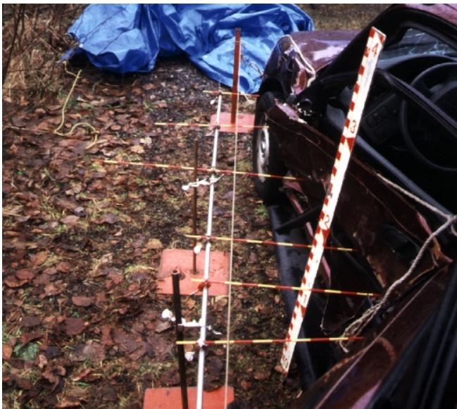
Figure C1 Side of a Pre-FMVSS 214 Passenger Vehicle after Collision with Another Passenger Vehicle
