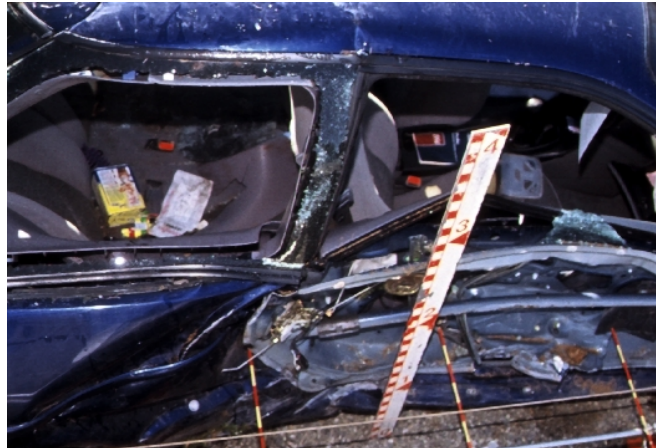
Figure C2 Side of a Post-FMVSS 214 Passenger Vehicle after Collision with Another Passenger Vehicle
