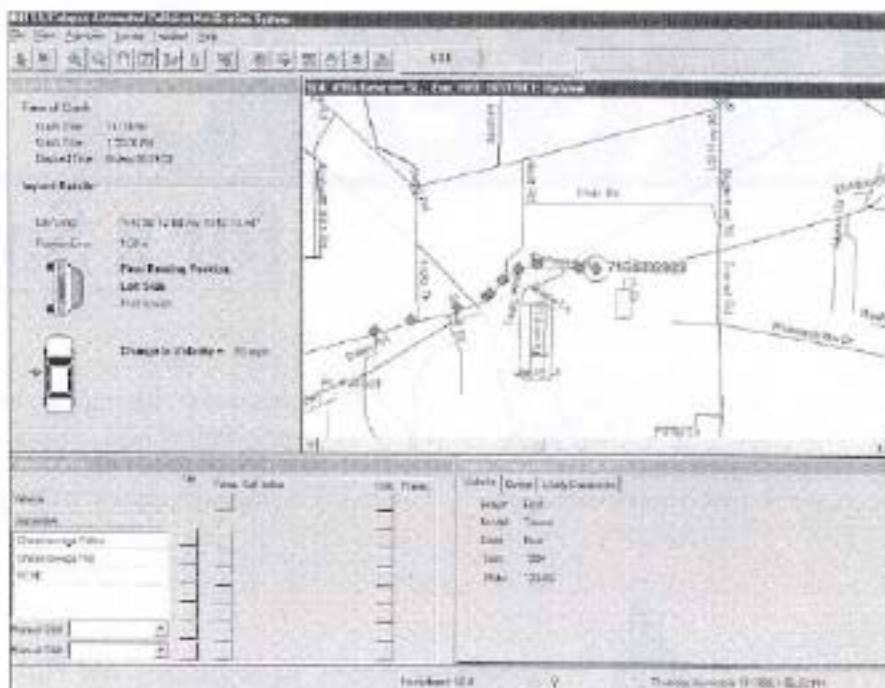
FIGURE 1. URGENCY software pinpoints the location and other vital details of vehicle crashes.
