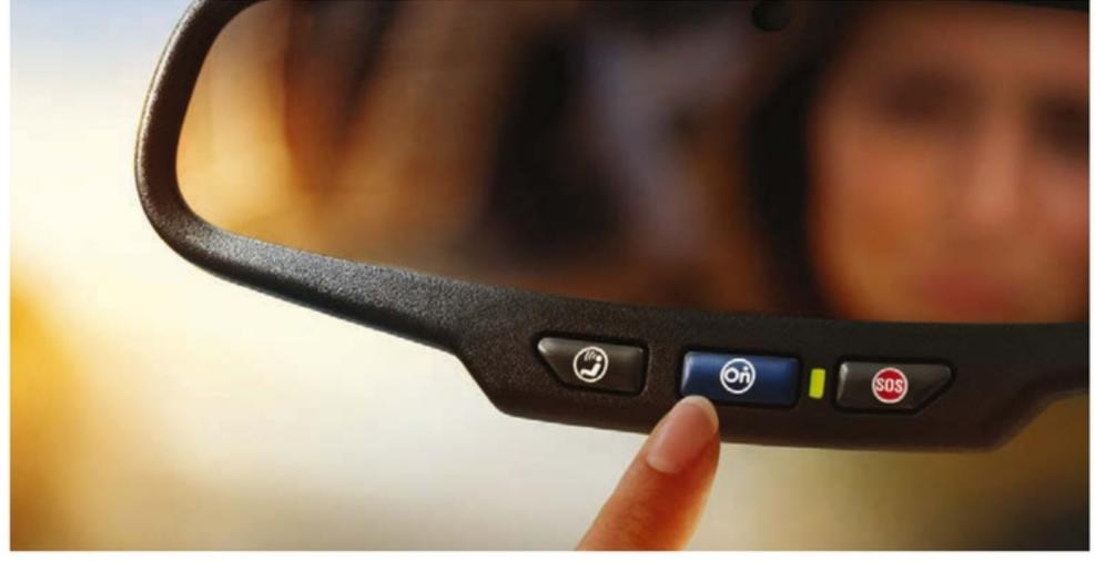
The call center approach enables GM to pass on detailed information to the emergency services about the nature and severity of the incident, gathered not only from talking to the victims, but also from the vehicle's sensors. OnStar users can also report other incidents on the road, and count on assistance in the event of severe weather and natural and man-made disasters.
